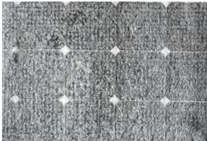
celle delaminate dal vetro delaminated glass cells
